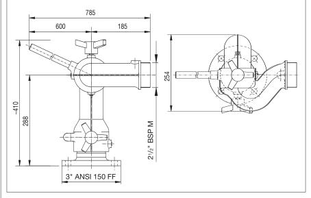
Note: when a large foam cannon is fitted a balance weight may have to be fitted to the monitor control handle.
