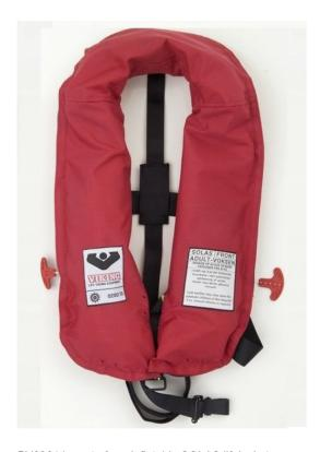
PV9361 is part of our inflatable SOLAS lifejacket range, which also includes PV9320 and PV9360. The lifejacket has a 275 Newton asymmetrical buoyancy chamber and can be configured with different types of buckles, covers, lights and inflation units etc., to fit customer specification. All features are trademarks with a proven performance record i.e. Cordura fabrics, ITW Nexus buckle system, Halkey Roberts and Hammar release units. The design of the lifejacket emphasizes both fit and performance.
